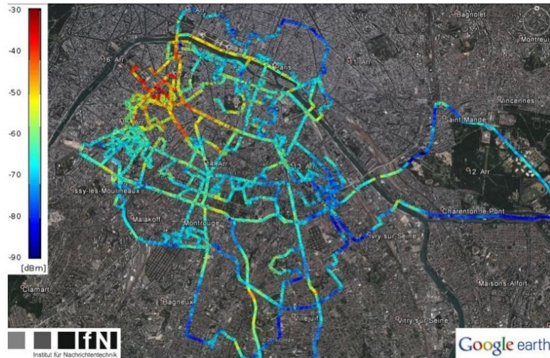
Figure 30: Overview of receiver input power levels measured during a field trial in central and south-eastern Paris Source:
